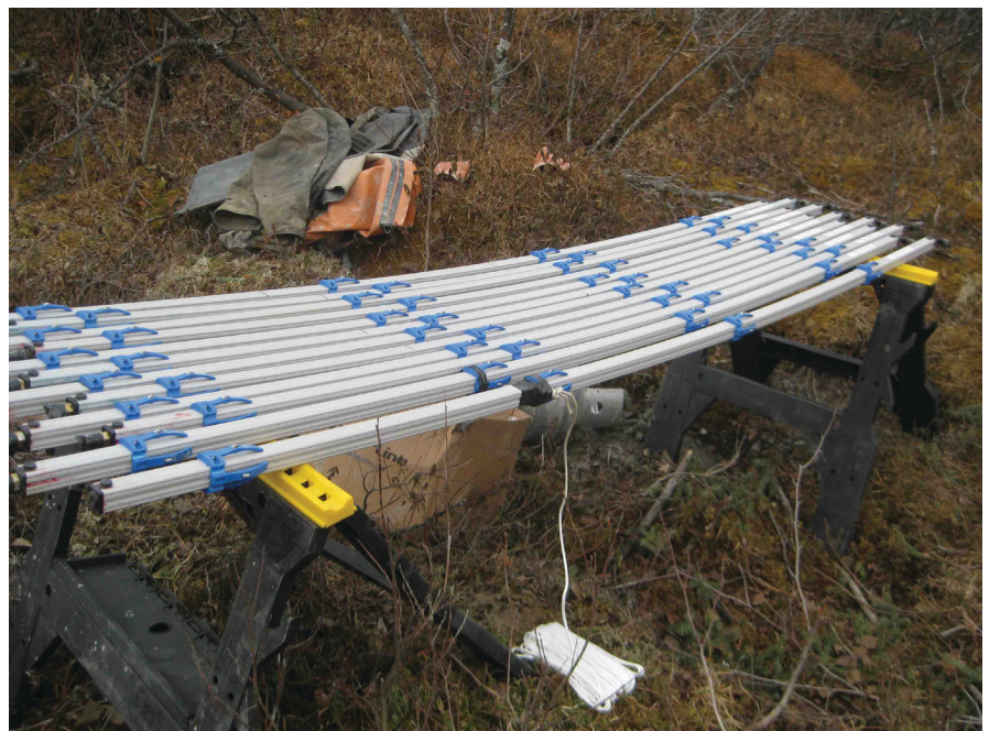
Figure 1. INC500 modules, staged with centralizers attached and ready for installation.
